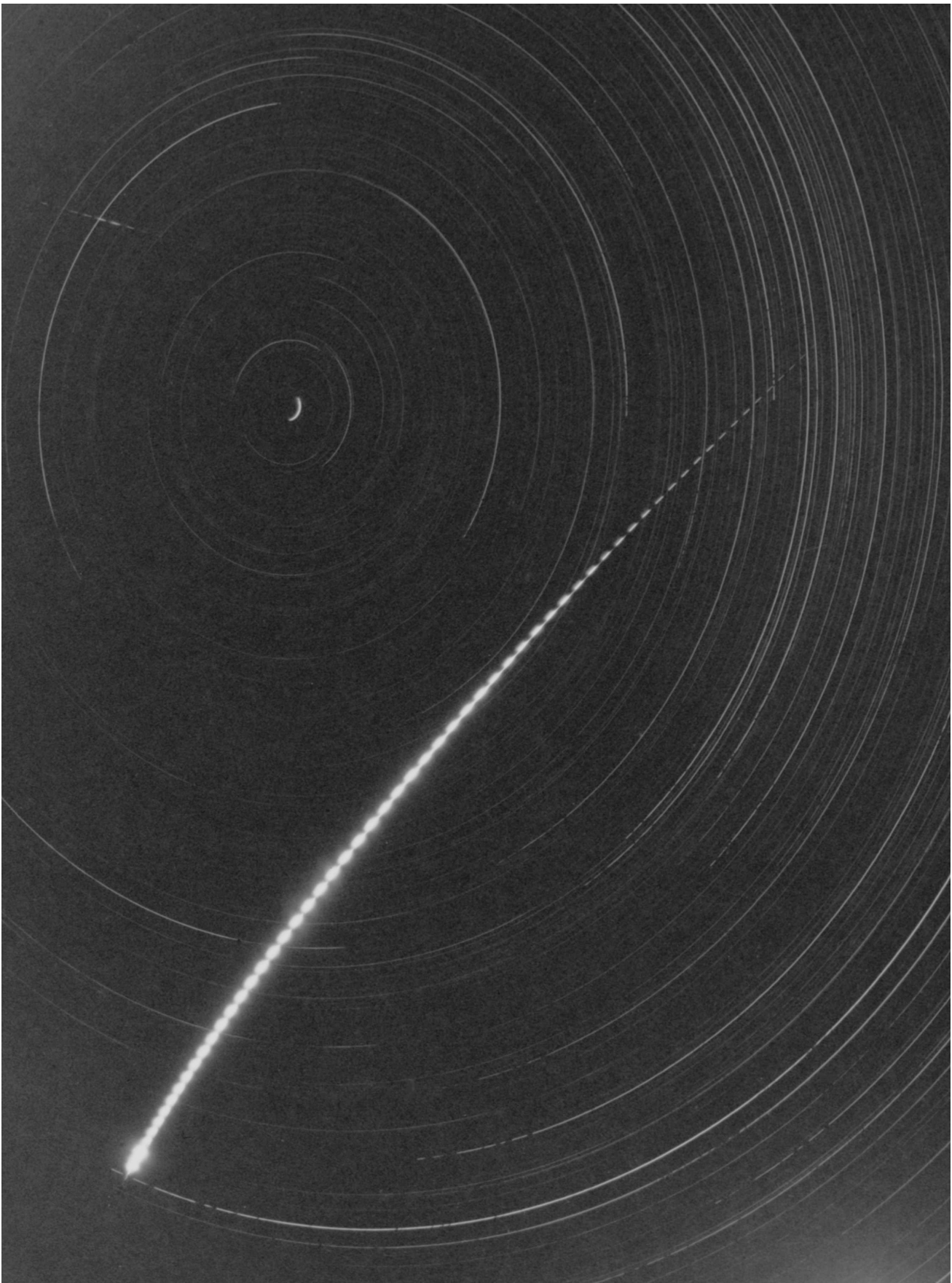
Figure 1 – Detailed view of the EN290903 fireball from the fixed all-sky camera placed at Lysá hora, the most eastern Czech station of the European Fireball Network. This camera is equipped with a Zeiss Distagon 30 mm f/3.5 fish-eye objective. Interruptions of the luminous path of the fireball are caused by a three-arm rotating shutter placed near the focal plane (15 breaks/s). The fireball started its luminous trajectory practically above the station, only 12 degrees far from zenith. The distance of the station from the terminal point was 77 km.
